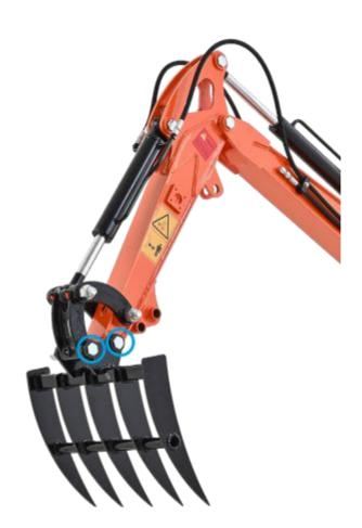
8. Restart the engine and test the rake by performing light operations to confirm its stability.
